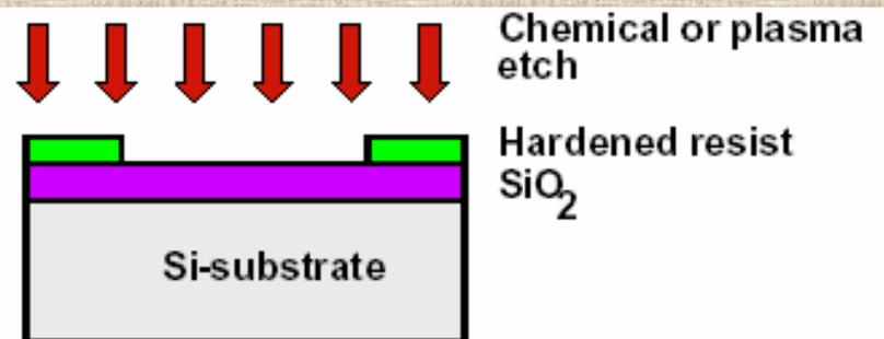
(d) After development and etching of resist, chemical or plasma etch of SiO<sub>2</sub>
