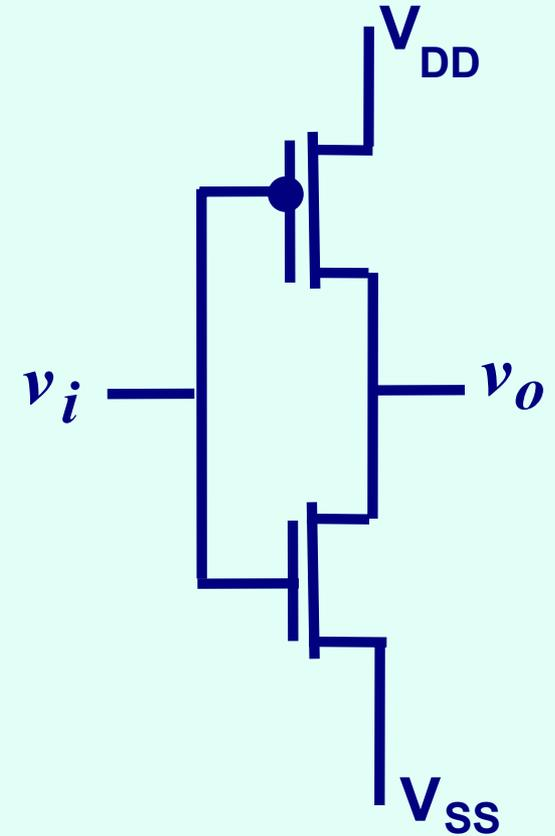
$$v_{GS_P} = v_i - V_{DD}$$
