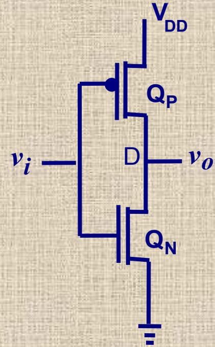
$v_{GS_N} > V_{T_N}$   $Q_n$  conduce
